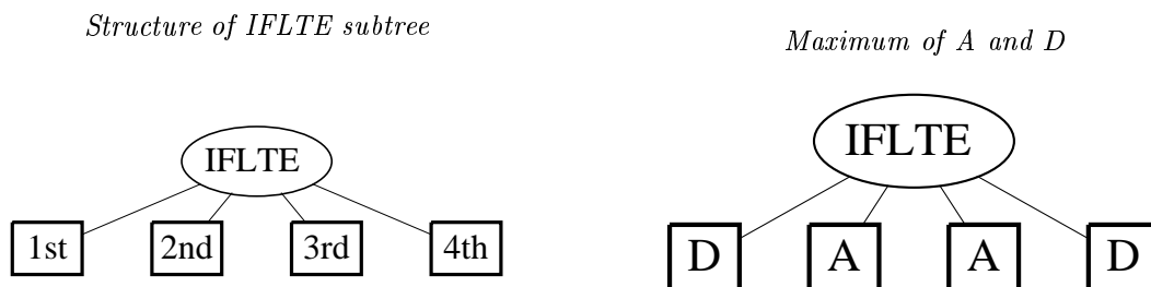
Figure 3.1: Structure of IFLTE subtree – ( If Less Than Or Equal to ), arity=4
