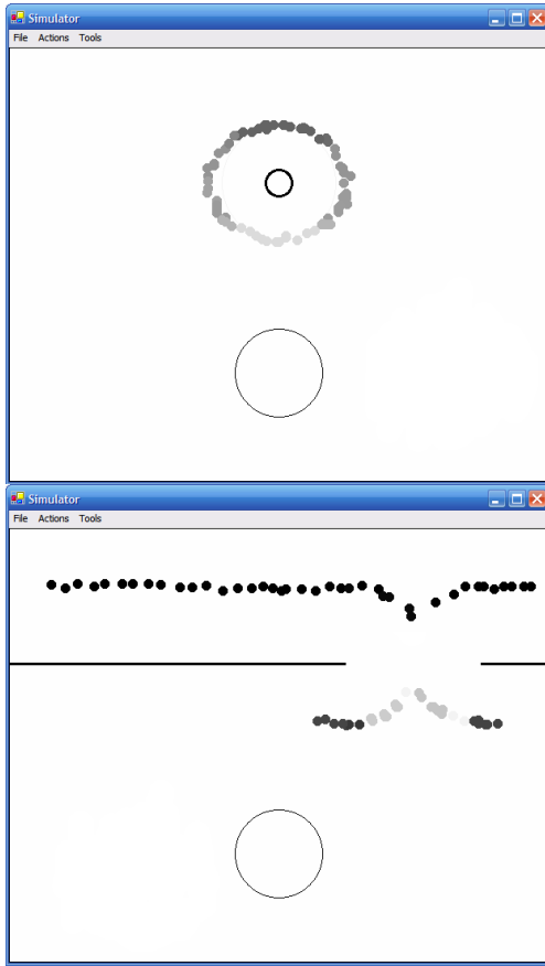
Fig. 3. RF for the skills constructed from the learned policy. All dots are final states and the color represent the reinforcement value (lighter colors for higher values).
