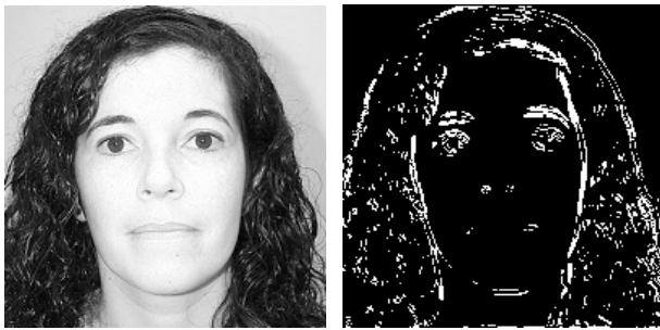
Fig. 7 – Example of first stage operation where a grey-level image (left) is transformed a binary image (right).
