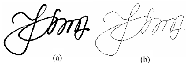
Fig. 2 – Signature (a) with its thinned version (b)
