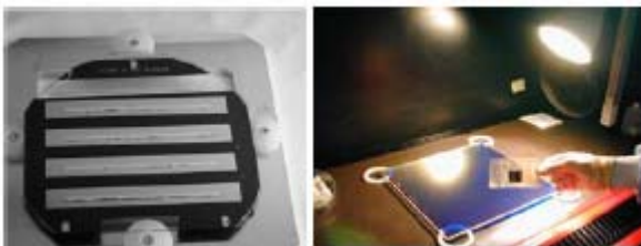
Fig. 7. Example of High-Tech optical devices performing optical filtering (left) and the visual fault detection, performed by an expert.
