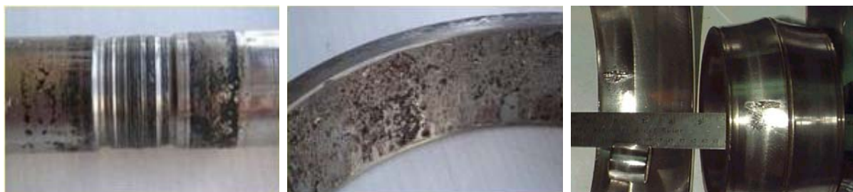
Figure 1: Examples of “Unbalanced Force Defect’s” effect on turning plant’s rotation axis (left) and “Flaking Path Defect” in a bearing device (middle and right).
