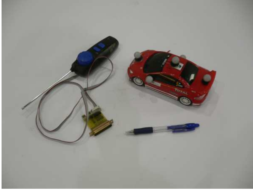
Figure 6.4: The toy car and its remote, note the reflecting markers.
