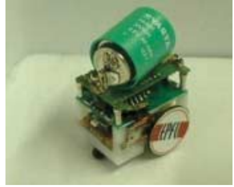
Figure 9: The mobile micro-robot Alice with the extra battery module providing up to 10 hour of energetic autonomy.
