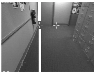
Figure 3: What is computed. For a given column of the image, the evolved vision subsystems compute the boundary between the ground (lower line) and a non-ground object (upper line). If there is more than one such boundary, the lowest is desired. This is done independently for six columns in the image.
