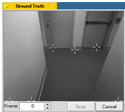
Figure 1: This program allowed the user to specify the lowest non-ground column in each image. The crosshairs could be moved vertically but not horizontally.
