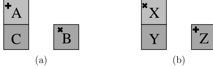
Figure 6.11. Deixis in a simple blocks world domain: The task in (a) is to place block B on A, while in (b) is to place X on Z. The two tasks reduce to that of placing block pointed to by \times over block pointed to by + .
