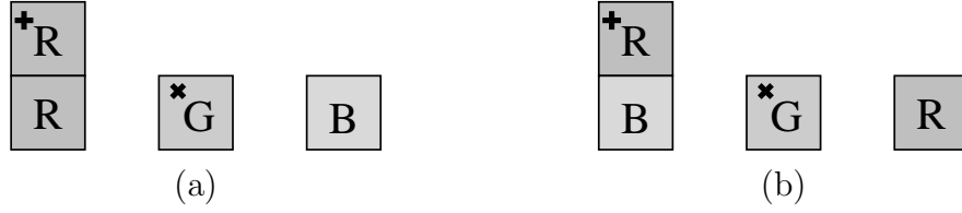
Figure 6.16. Perceptual aliasing in a simple blocks world domain: Both (a) and (b) map to the same representation and are treated as equivalent. But the task is to stack blocks of three different colors and the desired action in the two situations are different.
