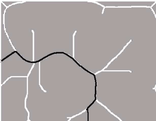
Fig. 9. Trajectory calculated with Fast Marching over the Voronoi Diagram of the Enlarged Laser data read by the robot (Local map).
