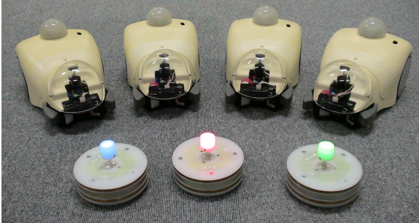
Figure 4.4. Four Cyber rodents and three battery packs with different colored (Red, Green, and Blue) LEDs mounted on top.
