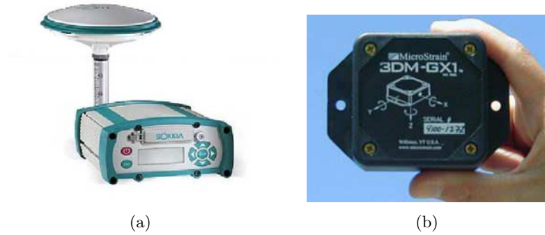
Figure 7: The Sokkia GSR2600 and Microstrain 3DM-GX1 sensors.
