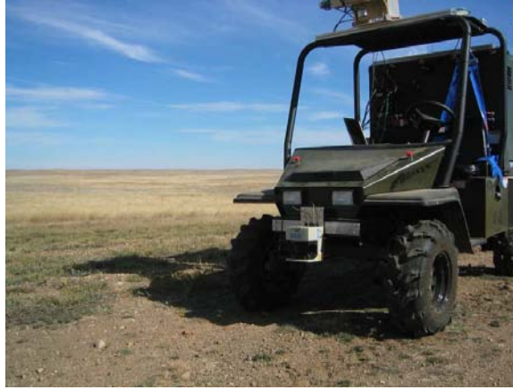
Figure 22: The laser mounting used for the VFH algorithm.
