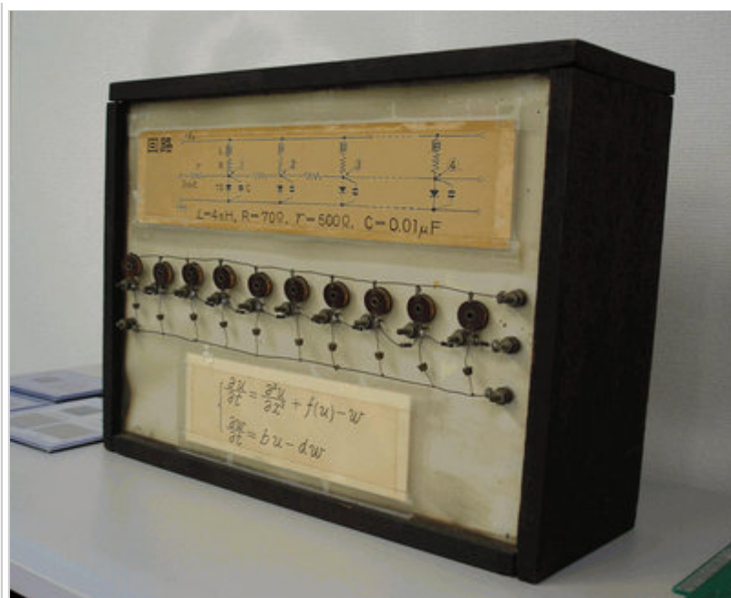
Figure 10: The original Nagumo circuit is held as a trust in the laboratory of Dr. K. Aihara in University of Tokyo. Photo provided by H. Suetani and K. Aihara with permissions.
