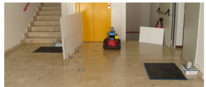
Fig. 12. Experimental set-up. The rover P3-AT facing an environment with two targets.
