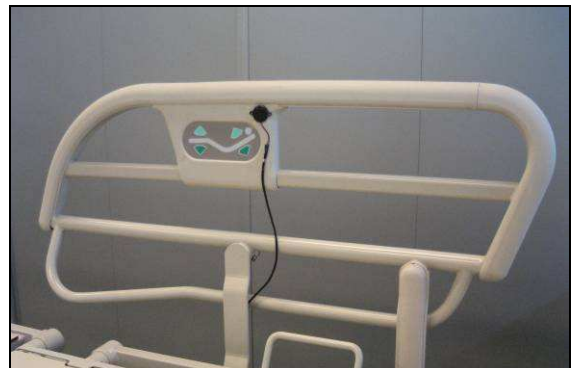
Fig. 6. Shock sensor installed in one of the bedrails.
