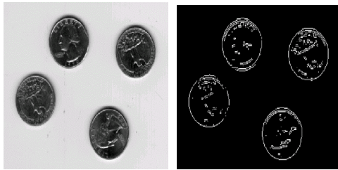
Fig. 3. (a) Original Coins Image;(b) After Averaging and Edge detection Templates by adapting RK-Embedded Contra-Harmonic Mean.
