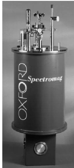
Figure 5.7: This is the Spectromag magnet. Ours is a maximum of 11.5 T magnet. The coils are located in the bottom portion and the upper portion houses a the liquid nitrogen bath and the vacuum space.
