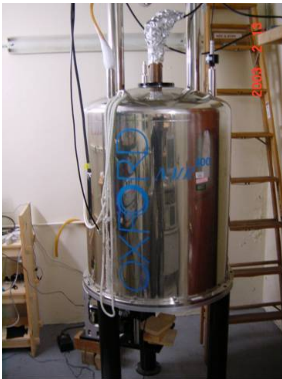
Figure 5.3: 7 T NMR magnet made by Oxford Instruments. We installed an optical breadboard below the magnet to mount the necessary optics. Aluminum supports screwed into holes on the bottom of the magnet. The laser and monochromator are located on a standard optical table and all the light to and from those equipment are fiber coupled.
