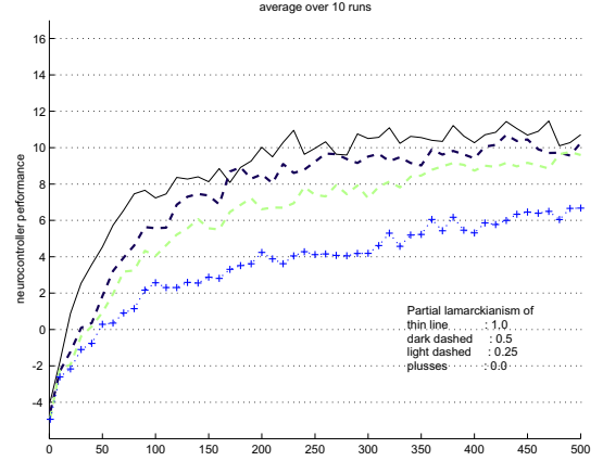
Figure 5: Neuro-controller performance plots for populations with partial lamarckianism. The fraction of the population to which back-coding is applied is varied from 0 to 1 (lamarck share).
